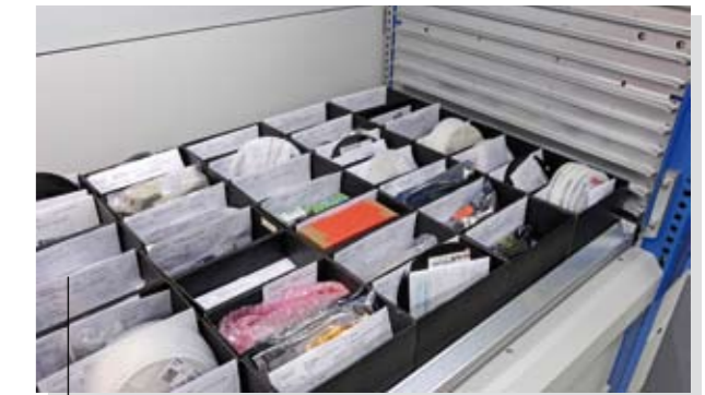
Tray with antistatic finish (ESD) for storage of the sensitive electronic material.
