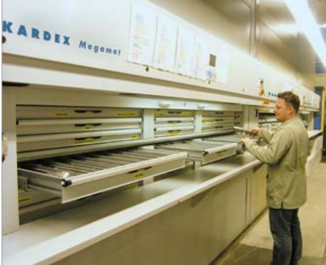
Kardex Megamat units replace racking for space-saving, ergonomic and efficient parts storage and retrieval
