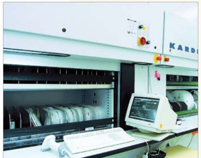
Special storage of rolled SMD components on the assembly line
