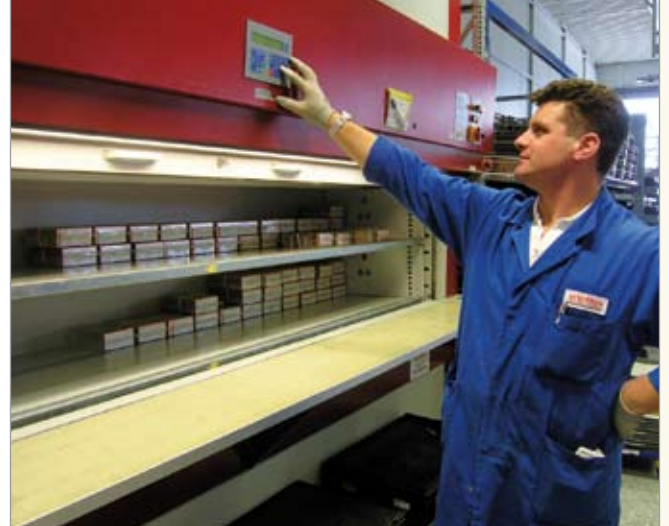
Storage of microchips with the ESD version as protection against electrostatic build-up
